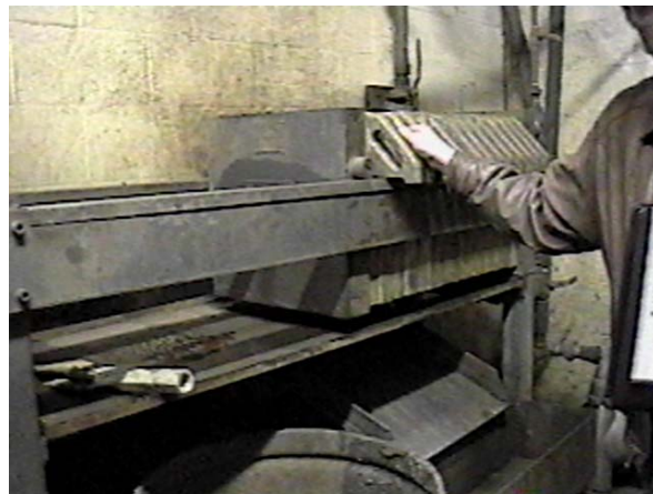
The screens in this filter press weigh 40 lbs and require cleaning every 2 hours
